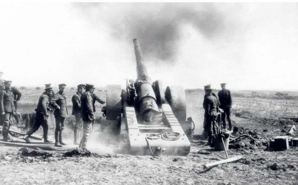
Firing a BL 6-inch Mk VII naval gun on a land carriage.
